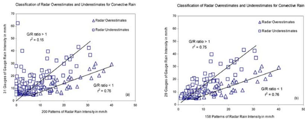
**Figure 2.** An example of G/R ratio for classifying radar overestimates and radar underestimates of convective rain. (a) The result after preliminarily justifying overestimates and underestimates. (b) The result after outlier elimination by the determination of correlation coefficient ( $r^2$ ) measure.
