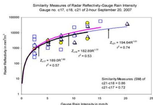
**Figure 6.** Similarity Measure (SM) of radar reectivity and gauge rain intensity of central gauge no. c21 and its neighboring gauges no. c18, c17 with SM of 0.86, 0.72. The Z-R relations are  $Z_{c21} = 194.64R^{1.61}$ ,  $Z_{c18} = 182.89R^{1.77}$  and  $Z_{c17} = 189.0R^{1.60}$  denoted by triangles, squares and circles symbols, respectively.
