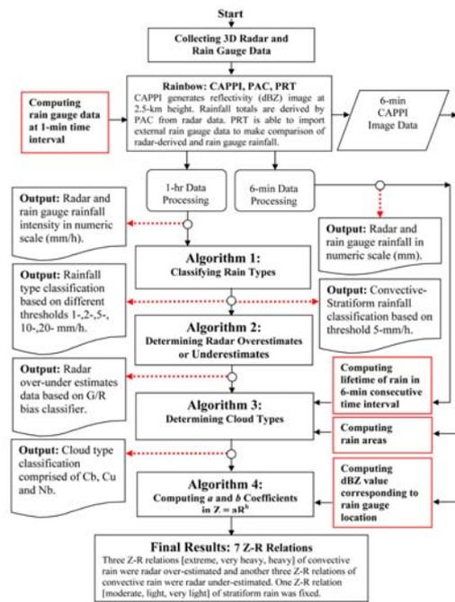
**Figure 1.** Algorithmic steps of our proposed technique. The thick lines denote the procedural flow and the dotted lines denote the outcomes of each step. The thick arrow denotes the flow of data to the next process and the dotted arrow denotes the flow of data to the reporting process.
