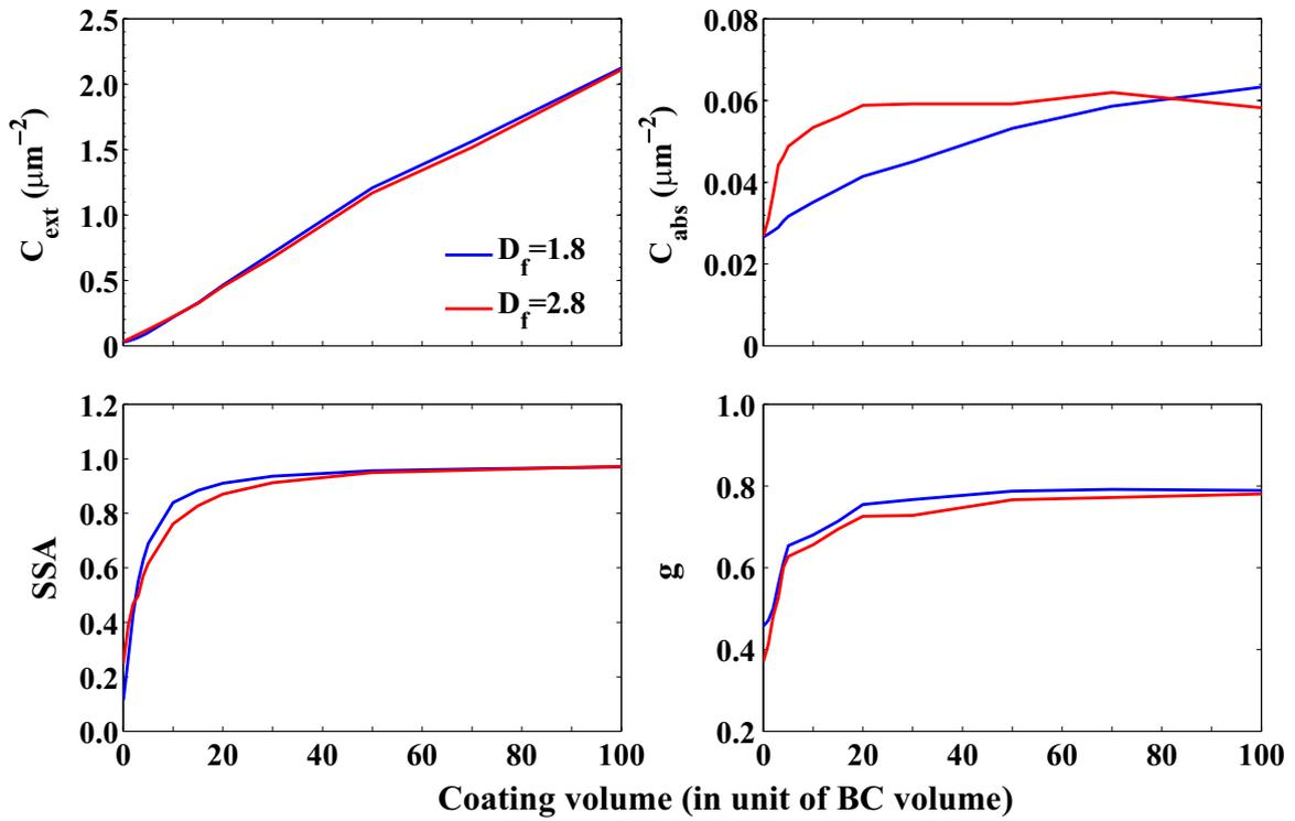
**Fig. 3.** Extinction cross section ( $C_{\text{ext}}$ ), absorption cross section ( $C_{\text{abs}}$ ), single scattering albedo (SSA) and asymmetry factor ( $g$ ) of BC aggregates with 200 monomers as functions of coating volume fraction.
