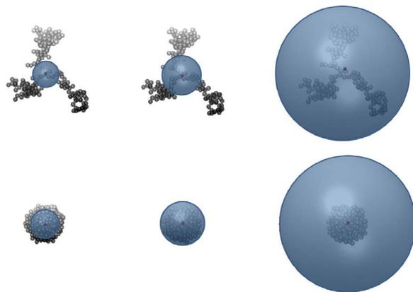
**Fig. 2.** Some examples of coated fractal aggregates with 200 monomers. The coating fractions from left to right are 0.5, 0.75, and 0.99.
