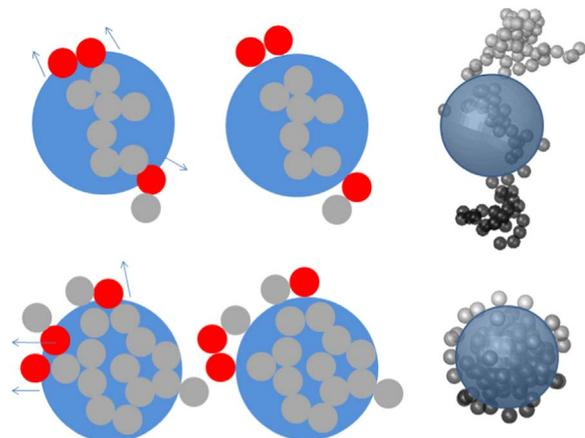
**Fig. 1.** Procedures to generate a fractal aggregate with a spherical coating and no overlapping monomers, and two examples of coated BC aggregates (100 monomers) with fractal dimension of 1.8 and 2.8. Gray and blue spheres represent BC and coating, respectively, and the red ones are the moved monomers. (For interpretation of the references to color in this figure legend, the reader is referred to the web version of this article.)
