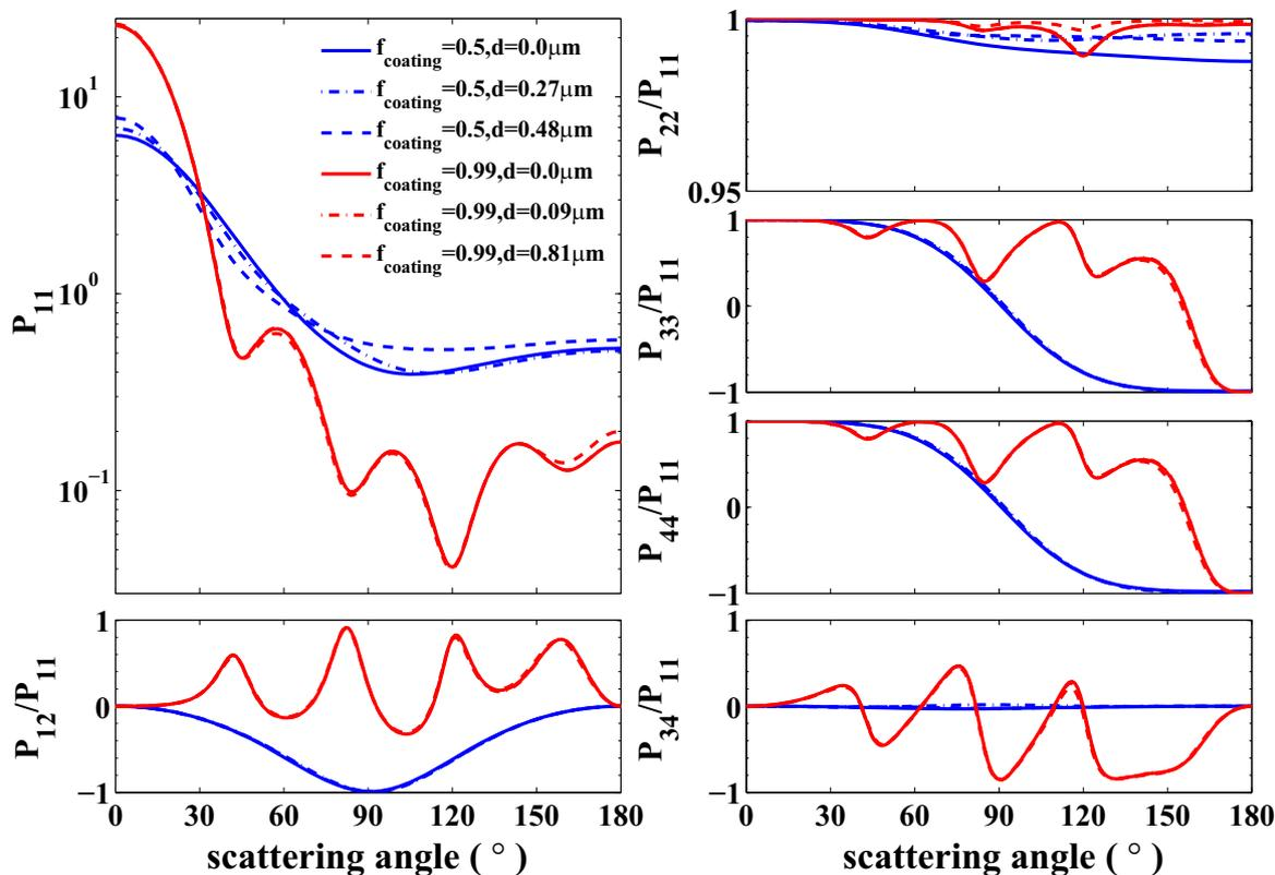
**Fig. 8.** Scattering matrix elements of BC aggregate with 200 monomers and non-absorptive coating, and the coating is located at the center, gyration radius and edge of the aggregate.
