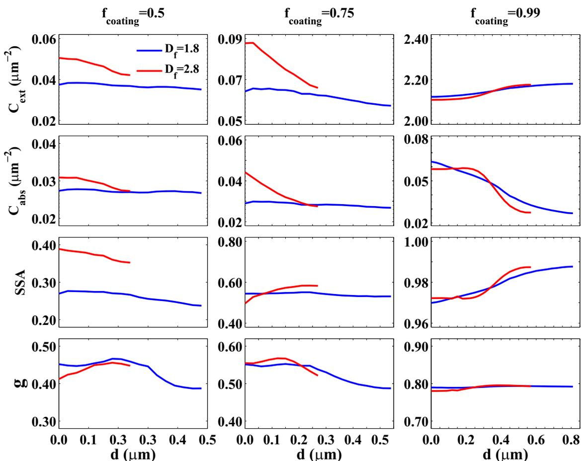
Fig. 7. Extinction cross section ( $C_{\text{ext}}$ ), absorption cross section ( $C_{\text{abs}}$ ), single scattering albedo (SSA) and asymmetry factor ( $g$ ) of BC aggregate with 200 monomers and different coating positions.
