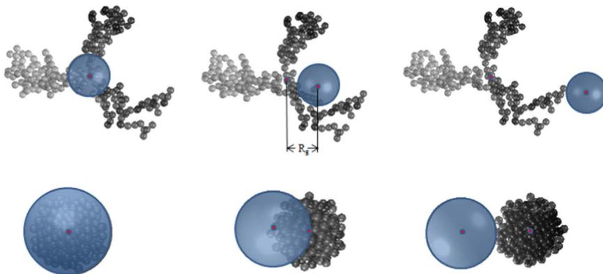
Fig. 6. Some examples of coated aggregates (200 monomers) with different distances between the aggregate and coating sphere.
