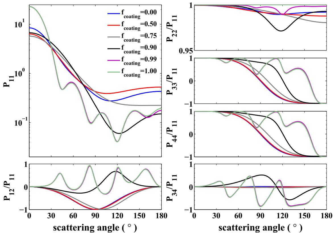
**Fig. 4.** Scattering matrix elements of BC aggregates with 200 monomers. The fractal dimension of the aggregates is 1.8, and the coating fractions of 0, 0.5, 0.9, 0.99 and 1.0 are considered.
